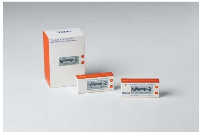
The August Faller Group has developed three prototypes for Smart Packaging solutions. These include – the “Level Indicator”, that calculates how much liquid remains in a bottle with fluid medication, the tablet counting “Counting Device” and the packaging “Medical Prescription” that not only counts the tablets and reminds the patients to take them promptly, but can also send the medication plan via Bluetooth to the packaging, using a specially developed app.
